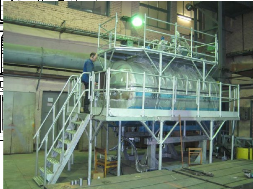
Fig.1. Gravitational spectrometer with service platforms
